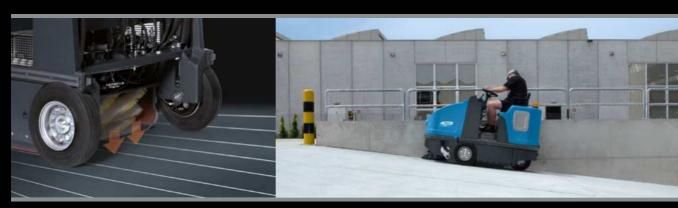
The central brush is the floating type and self-adjusts to keep in contact with the ground all the time
